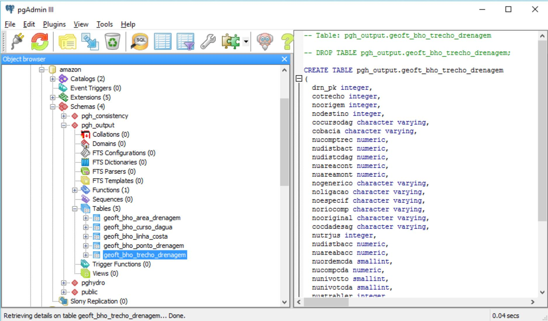
The screenshot shows the pgAdmin III interface. On the left, the Object browser displays a tree view of the database structure. The 'amazon' database is expanded, showing 'pgh\_output' as a schema. Under 'pgh\_output', the 'Tables (5)' folder is expanded, and 'geoft\_bho\_trecho\_drenagem' is selected. The main SQL editor on the right contains the following SQL code:
